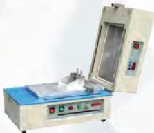
Tape casting and roller pressing to preparing electrode film
