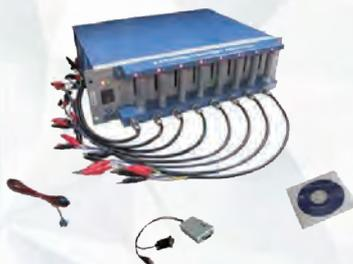
Test of coin cell and split coin cell with computerized precision battery analyzer (0.002 mA – 3000 mA)
